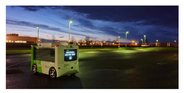
Finally, Valeo eDeliver4U brings together plug & play visibility, lighting and signaling systems that are immediately ready to use. The goal is multifaceted: keep sensors operational no matter the conditions [*see technical details below*]; let the droid see and be seen by everyone, especially pedestrians; and communicate using HD-resolution screens, with people interacting with the droid.
