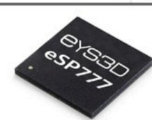
eSP777 - Dual Fisheye Lenses 3K2K Stereo Dewarp/Stitch Processor
